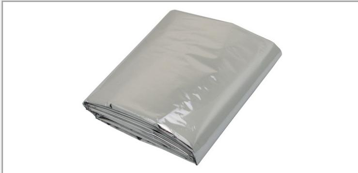
Made of polyethylene (PET) and aluminium. Size: 200 x 120cm. Thickness: 12 microns. Keeps 90% of heat radiation. 1 silver surface / 1 gold surface. Silver surface on the outside: reflects heat rays and isolates from heat (effective air conditioning for a tent, caravan or car). Gold surface on the outside: isolates from moisture, cold, and rain (in case of an accident, helps maintain body temperature).
