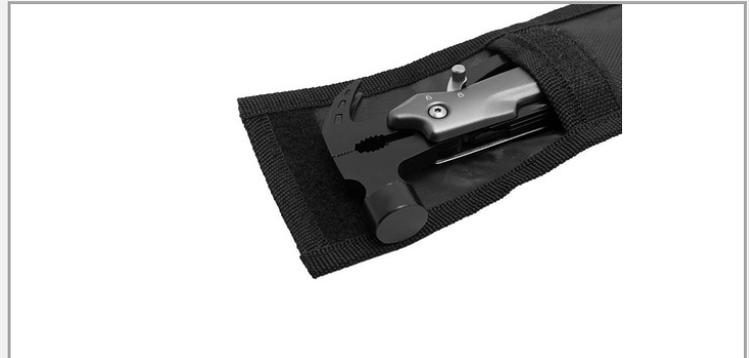
Professional multifunctional hammer made of highly resistant 420 stainless steel. Aluminium handle. New generation safety lock (easy unlocking). Torx screw assembly. 11 functions: hammer, universal pliers, cutting pliers, knife, saw, scissors, file, bottle opener, nail puller, Phillips screwdriver, flat screwdriver. Rockwell hardness: 48 degrees. Heather grey 420D nylon belt pouch included.
